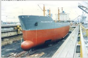
5.5: Ship on Sun Ship's No.4 Dry Dock undergoing final hull work and painting prior to delivery-Aft View SSHS: 500\_677\_04a<sup>1</sup>
