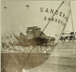
IRRESISTIBLE FORCE (above) met IMMOVABLE OBJECT (below) with result as shown. Norwegian tanker Sandefjord and barge owned by C. J. Willis Co. were in collision in Delaware and had not far to go for repairs. Barge is coastwise, deckhouse, cargo barge, one of largest on eastern seaboard.
