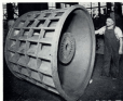
ONE EXAMPLE of one of the unusual products made in our Foundry is this 48 inch diameter steam shaft which after machining by Westport was installed in a Merchant plant.
