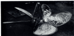
ONE PROPAN and turbine inlet valve and various hot shaft and turbine components all come through manufacturing from the Machine Shop, the same as for that 304 inch pipe, this turbine propeller, approximately 24,000 lbs., was produced and actually finished for length. It will be shipped to Westport by water due to its 24 1/2 diameter.
