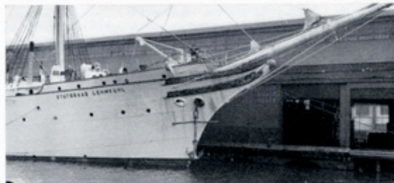
LIKE THE CLIPPERS OF OLD, this view shows her raking bowsprit and fine lines. The stack behind the foremast is for the auxiliary diesel which is used for maneuvering in narrow channels.
