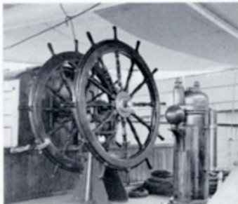
THE SHIP'S WHEEL. In bad weather the wheel is more than one man can handle. Sometimes four men are needed.
