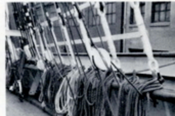
VIEW SHOWING THE MAZE of running rigging. Working in the dark, a windjammer seaman can lay his hand on any stay, line, tackle, sheet, shroud, halyard, etc. shown here.
