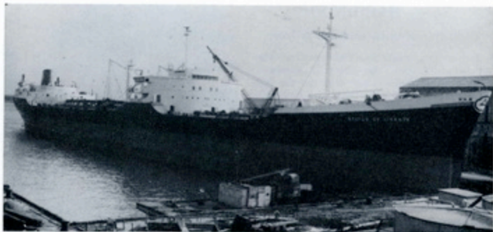
THE 707 STATUE OF LIBERTY, in yard for boiler repairs, is the longest merchant ship ever in the yard. One of four sister ships, she has a 93' beam with 48' 6" depth, can carry 38,000 DWT with a barrel capacity of 336,000; does 17 1/2 knots on 20,000 h.p. The aircraft carrier Ranger, scrapped in our yard, measured 769' long.
