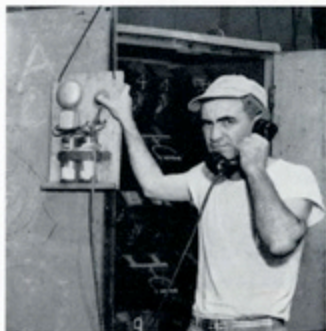
(Above)— JOHN LOGUE operating load boxes on dock for load test. He gets his instructions by phone from the engine room.
