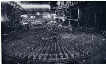
OUR SHOP'S GARDEN in heavy industrial equipment is illustrated by the 24' diameter grid support at (foreground) for a large oil refinery.
